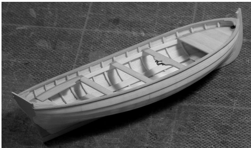
Gunwale, breast hook and transom knees completed
